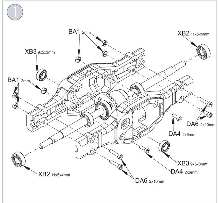
Ball bearing Kugellager
