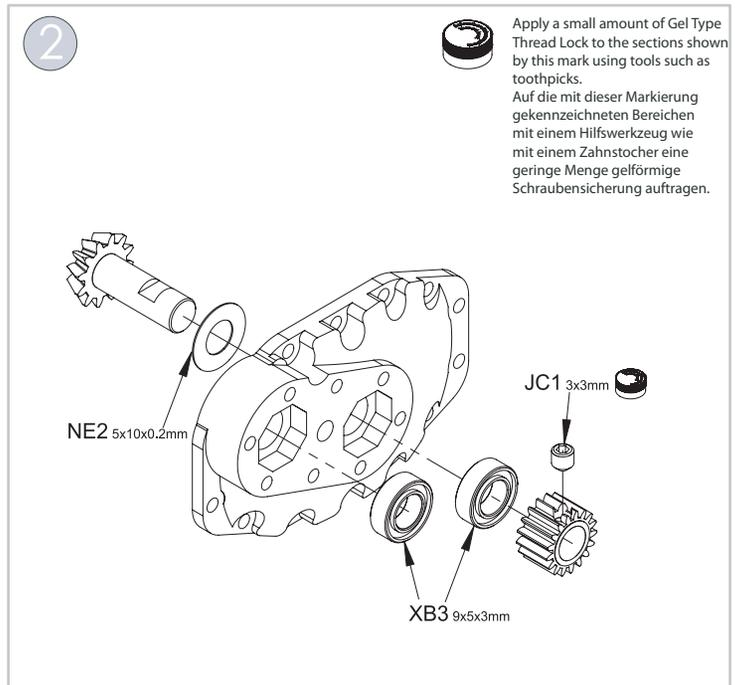
Apply a small amount of Gel Type Thread Lock to the sections shown by this mark using tools such as toothpicks.
